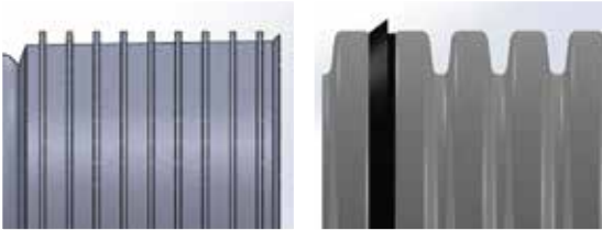
Sealing Rubber Ring Placement with orientation
